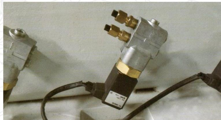
**One by two solenoid valve control weft insertion.**
