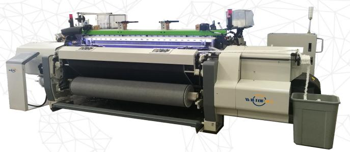
Type HYRL-1739 High Speed Rapier Loom, as a leading weaving machine, following market demands and development, is designed to weave high quality, high value-added fabric, with the features of advanced technology, reliable structure, easy maintenance, high-speed and high-grade.
